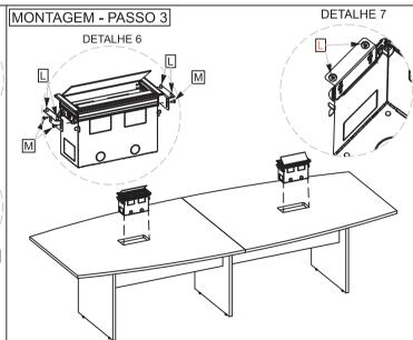
PARA FINALIZAR A MONTAGEM, ENCAIXE A CAIXA BASIC (K) NOS TAMPOS E FIXE OS SUPORTES LATERAIS NA CAIXA CONFORME O DETALHE 5, PARA QUE MESMA POSSA SER FIXADA NOS TAMPOS (1) CONFORME INDICA O DETALHE 7.
